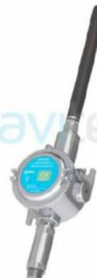
WSLRWEX-PPS is the LoRaWAN Integrated Process Pressure Sensor with Exd approval for installation in Zone 1, Zone 2 or Safe Zone, and it has different kinds of measurements, such as Gage/Absolute/Sealed Gage, range -1 .. + 1000 bar, high accuracy, and stability. With Ultra-low-power design and smart firmware allow the sensor can last up to 10 years with a single C battery (depending on configuration). It can support all LoRaWAN frequency bands in the World.
